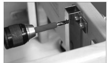
Figure J: Drill through receiver and into Reformer until drill bit hits the inside face of the mounting plate.
