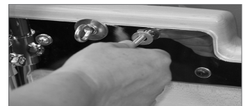
Figure H: Install the bolt and washer from outside of frame.
