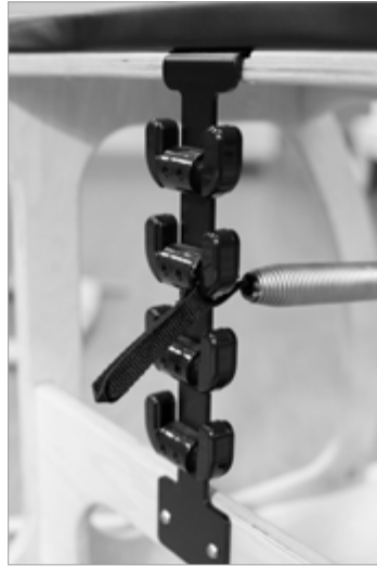
"Chair Cactus" attachment point found on various Chairs. It may also be flatter and made of sheet metal.
